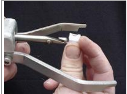
Load clip w/ notch up and forward.
