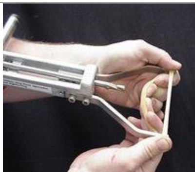
Start stretching lower portion of band with remaining fingers.
