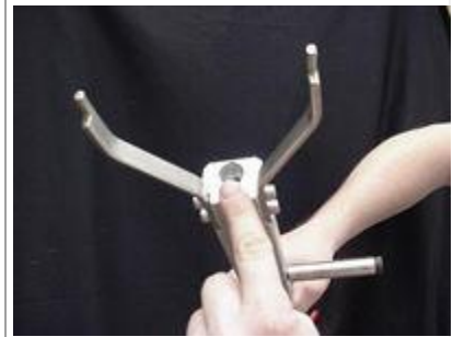
Place clip in slot so it is completely in and flush.
