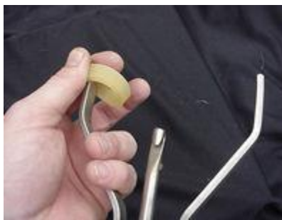
Hold band with thumb on top & index finger on end of spreader bar to keep from slipping off.
