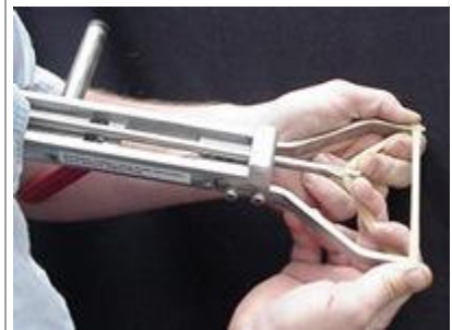
Continue until band is in groove of pull back rod.
