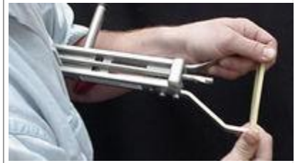
Hold band with both thumbs on top and both index fingers in the end of spreader bars.
